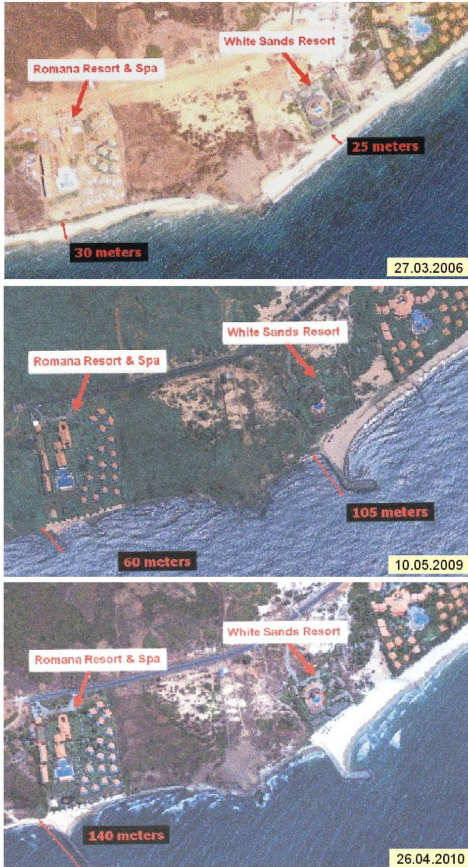
**Fig. 6:** Evolution of the beach erosion and consecutive construction of jetties for protection, first in front of the White Sands Resort (2009), then in front of the Romana Resort & Spa (2010). For location, see: Fig. 3[b]
