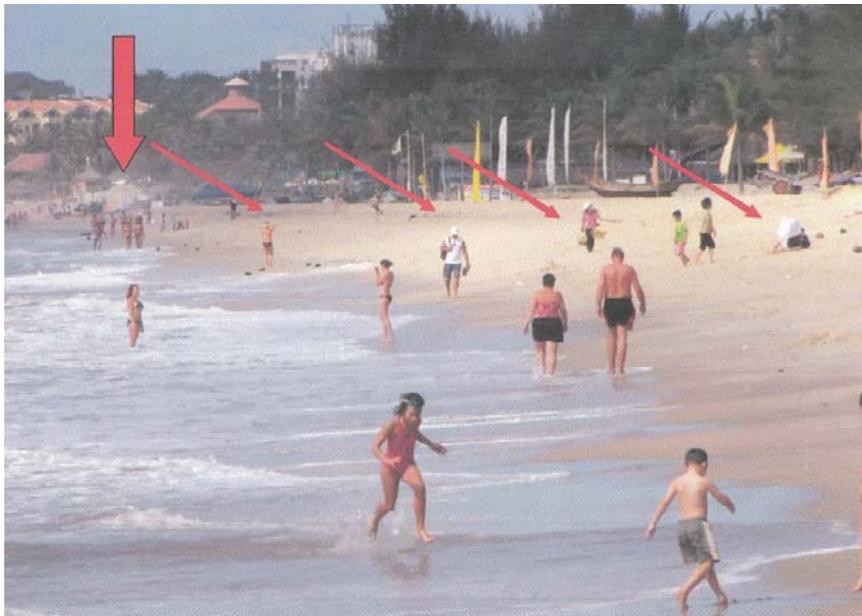
**Fig.11:** Artificial refill of beaches. Sand comes by truck (large arrow on left), then distributed on the beach on a daily basis in order to slow erosion
